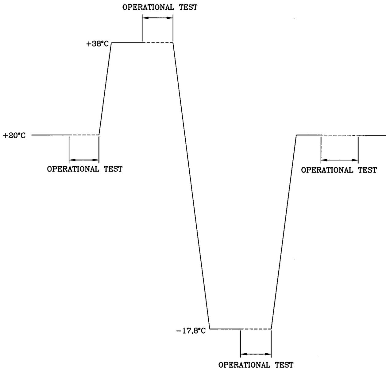
Fig.3a Environmental cycle extreme for 18 mm assembly
