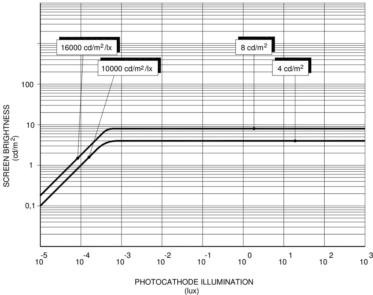
Fig. 5 Phosphor emission characteristic
