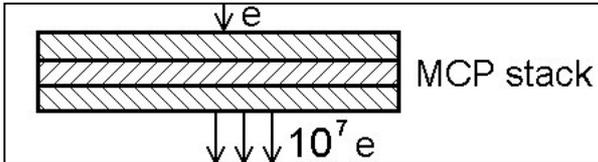
**Figure 12. MCP amplification**
