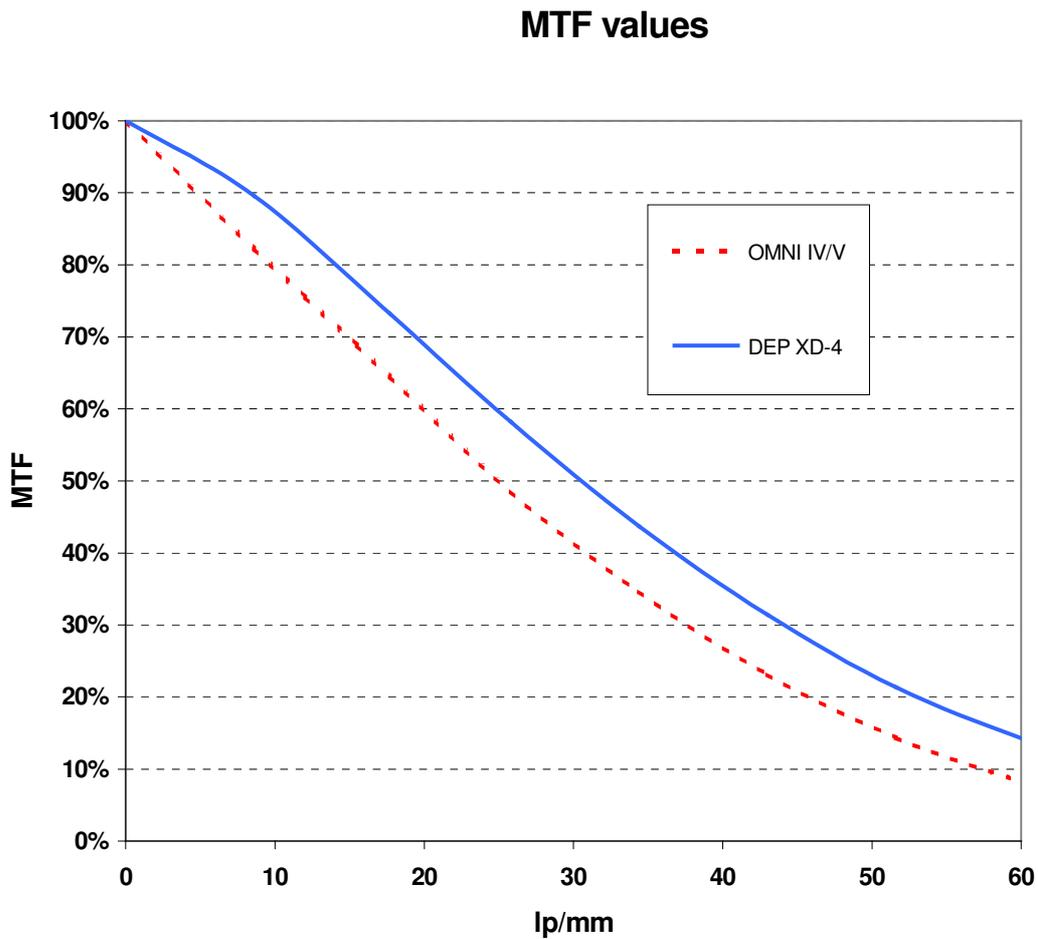
**Figure 7.** The MTF of Omnibus IV/V and DEP XD-4™
