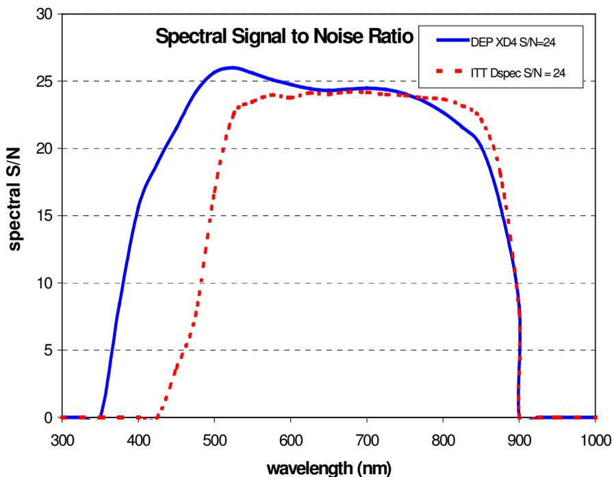
**Figure 6.** The spectral signal to noise curve for XD-4™ and GEN III, Omnibus IV/V.
