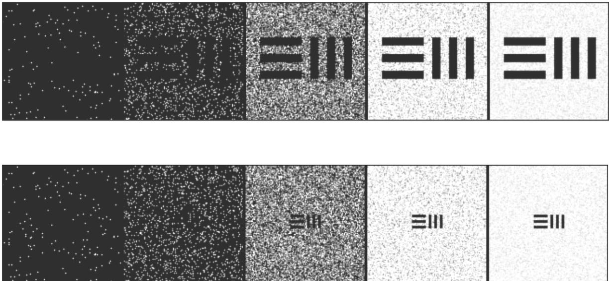
**Figure 2.** The 20 lp/mm and 60 lp/mm targets at different light levels
