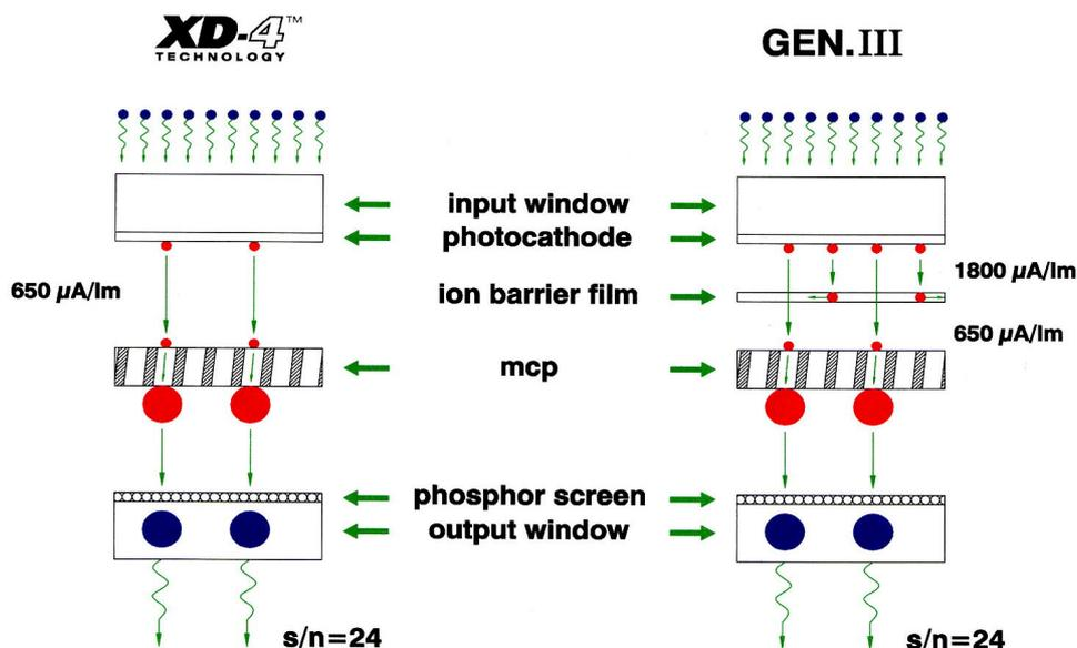
**Figure 3.** Visualisation of the difference between XD-4 and GEN III
