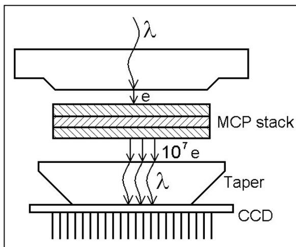
**Figure 14. MCP amplifier with CCD read-out**
