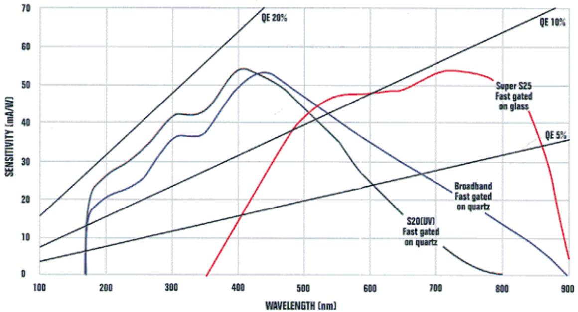
**Figure 11. Photocathode types (fast gated)**
