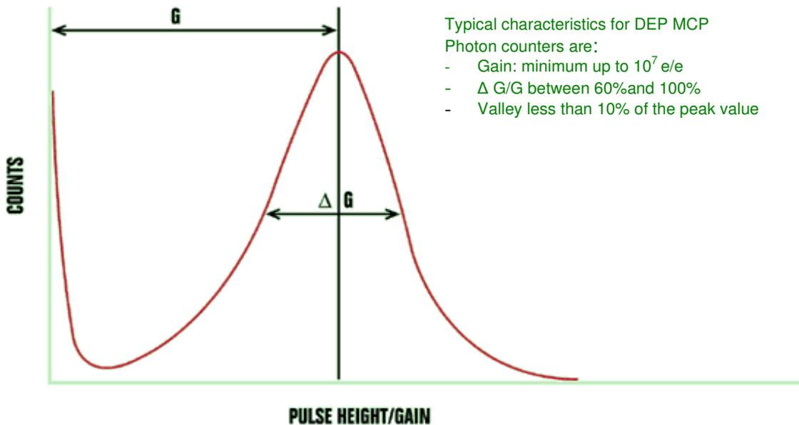
**Figure 13. Saturated Pulse Height Distribution for MCP photon counters**
