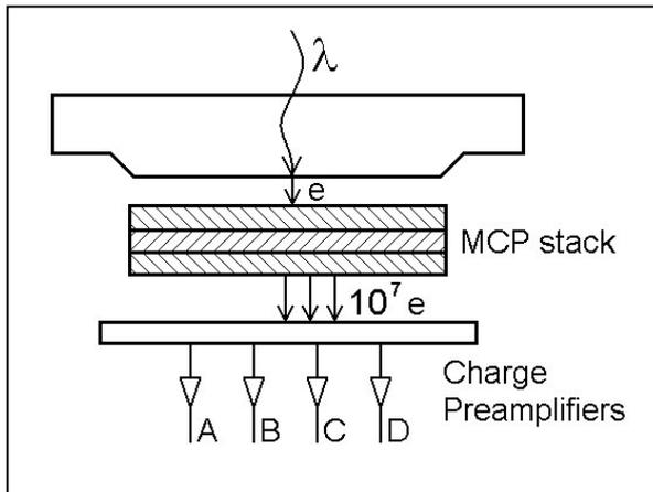
**Figure 15. Resistive anode intensifier**
